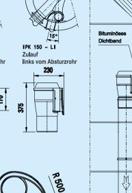
The IPK enables connections up to a pipe outer diameter of OD 180mm.
