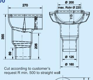
The INSIDE FUNNEL 200 enables connections up to a pipe outer diameter of OD 220 mm. The outlet offers two different diameters, either of OD 125 mm or OD 160 mm. The radius is cut at the factory to match the manhole wall.
