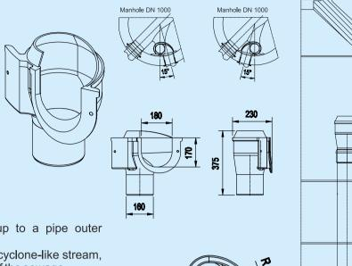
The IPK enables connections up to a pipe outer diameter of OD 180mm.
