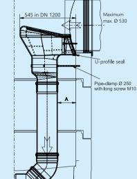
Straight wall = 120 Manhole Ø 1200 = 185 Manhole Ø 1500 = 170 Manhole Ø 2000 = 160
