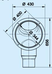
The Inside Drop Type 1 enables connections up to a pipe outer diameter of OD 330 mm. The maintenance / inspection access (220 mm) is closed with a screw-on cover. The outlet offers two different diameters, either of OD 160 mm or OD 200 mm. The radius is cut at the factory to match the manhole wall.
