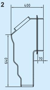
The Inside Drop Type 2 enables connections up to a pipe outer diameter of OD 375 mm. The maintenance / inspection access (approx. 288 x 221 mm) is not closed. The outlet offers three different diameters, either of OD 160 mm, OD 200 mm or OD 250 mm. The radius is cut at the factory to match the manhole wall.
