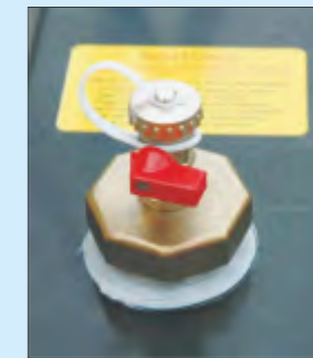
Before opening the screw of the pressure valve check for high pressure
